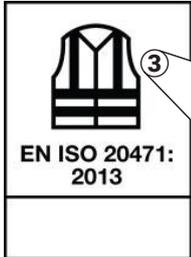
**ISO 20471:2013 High-Visibility Clothing** is an international standard which specifies requirements for high visibility clothing capable of visually signalling the user's presence.
