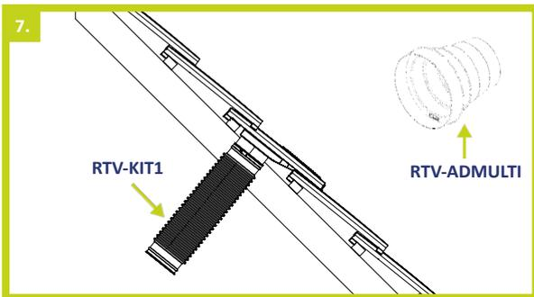
7. To connect the tile vent to a mechanical ventilation system or soil stack connect ductwork directly to the base of the tile vent or via the **RTV-KIT1** 110mm Flexi-Pipe kit. The **RTV-ADMULTI** stepped duct adapter can also be used and cut to size to accommodate various duct diameters.
