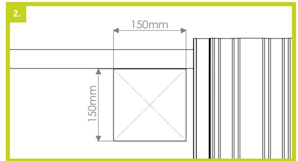
2. Mark out a rectangular area on the underlay just below the batten 150mm (W) x 150mm (H). Now mark a cross shape through the centre of the rectangular area to guide when cutting the underlay.
